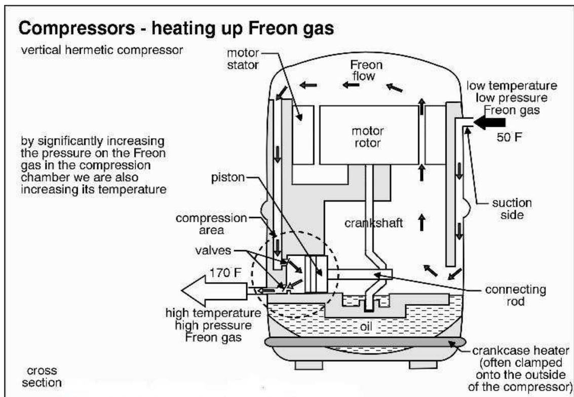
**A regular air conditioning system uses the compressor** to increase the pressure on the gas, heat the gas, than sends it to the condenser where it becomes a liquid again through the use of the condenser coil. The change of state of the refrigerant, starts to take place approximately 2/3rd's of the way down the condenser.
