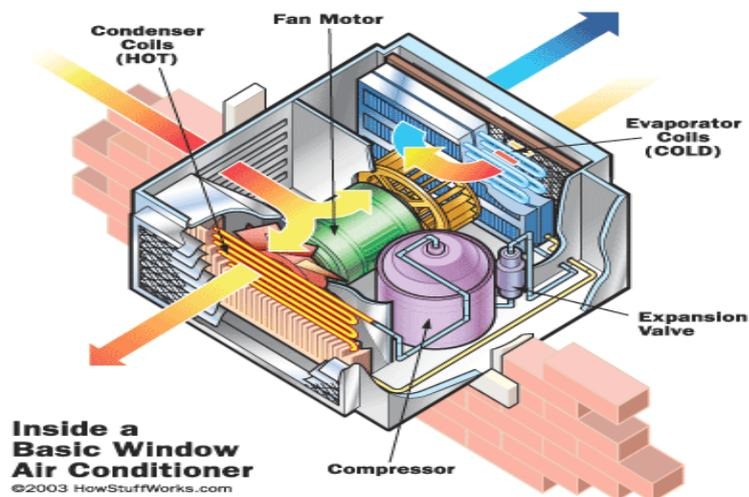
The working fluid leaves the compressor as a hot, high pressure gas and flows into the condenser.
