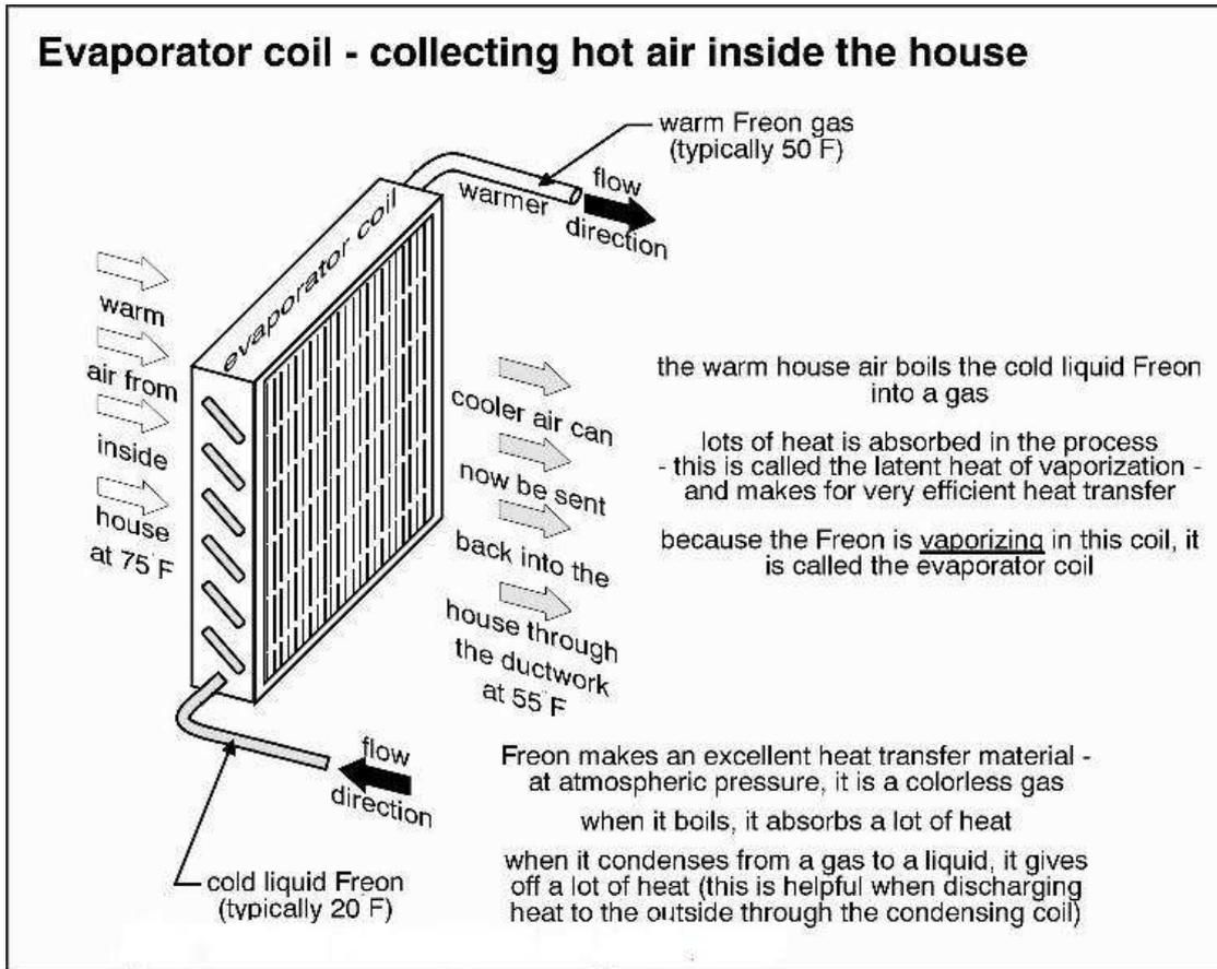
**This is where the cooling takes place...** all the rooms warm air heat is drawn into and passed through the evaporation coil...the evaporating of the liquid with a very low boiling point has done the job of removing this heat and the cooler air is sent back into the room.
